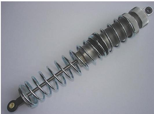
Step 13: Complete the shocker with applying springs. With dual springs, make sure to use the smaller spring on top. Dual springs are seperated by a spring splitter.
