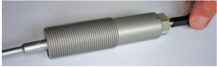
Step 7: Push the piston rod fully into the housing. Assemble now the ring-piston-ring and secure with the nyloc nut.
