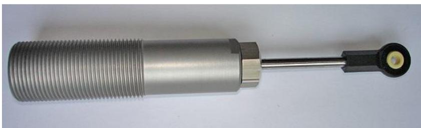
Step 6: Lubricate the top of piston rod with a bit of silicon oil. Place piston rod into the shocker housing from the bottom. When passing the seal rotate the piston rod and gently push through the seal. Never mount the piston rod from the other direction!
