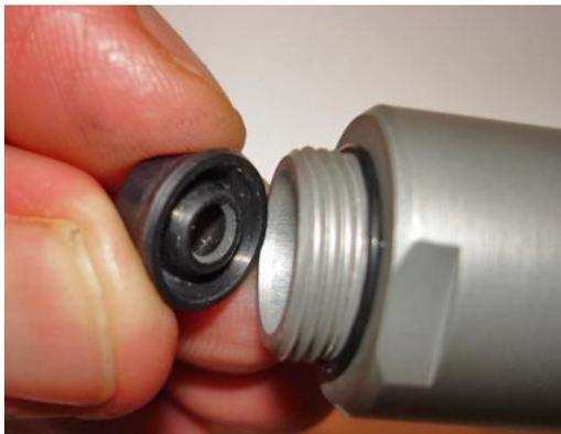
Step 1: Place the smallest o-ring around the housing over the thread.
