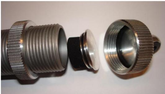
Step 12: Fill shocker with oil. Depending on shocker type 3~6mm under the edge. Let air escape while moving the piston gently up and down, keep the piston under the oil surface. Place lid till it sits on the o-ring. Move up the piston until 3/5<sup>th</sup> compression, oil should bleed out. When not bleeding, shocker was insufficient filled with oil. Now push in the lid and at the same time pull the rod out. Remove oil on outside of housing and assemble the top cap.
