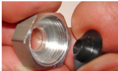
Step 3: Place dirt scraper inside the closing cap for the bottom.
